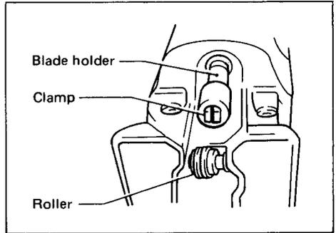
5. With the blade installing knob kept in this position, push it back down to its original position.
