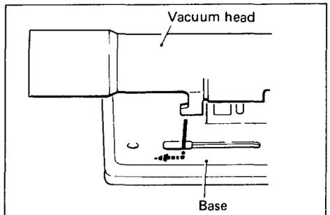
To attach the vacuum head on the tool, insert the hook of the vacuum head into the hole in the base. The vacuum head can be installed on either left or right side of the base. Then connect a Makita vacuum cleaner to the vacuum head.
